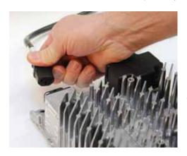
Figure 1: Disconnect AC input from the charger.
